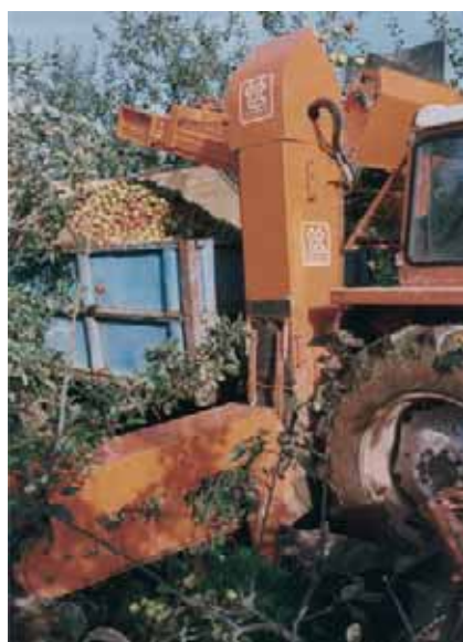
Centipede harvester in 5.5 metre row
