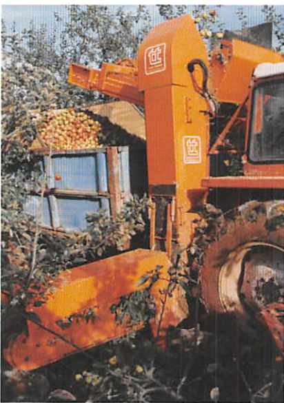
Centipede harvester in 5.5 metre row
