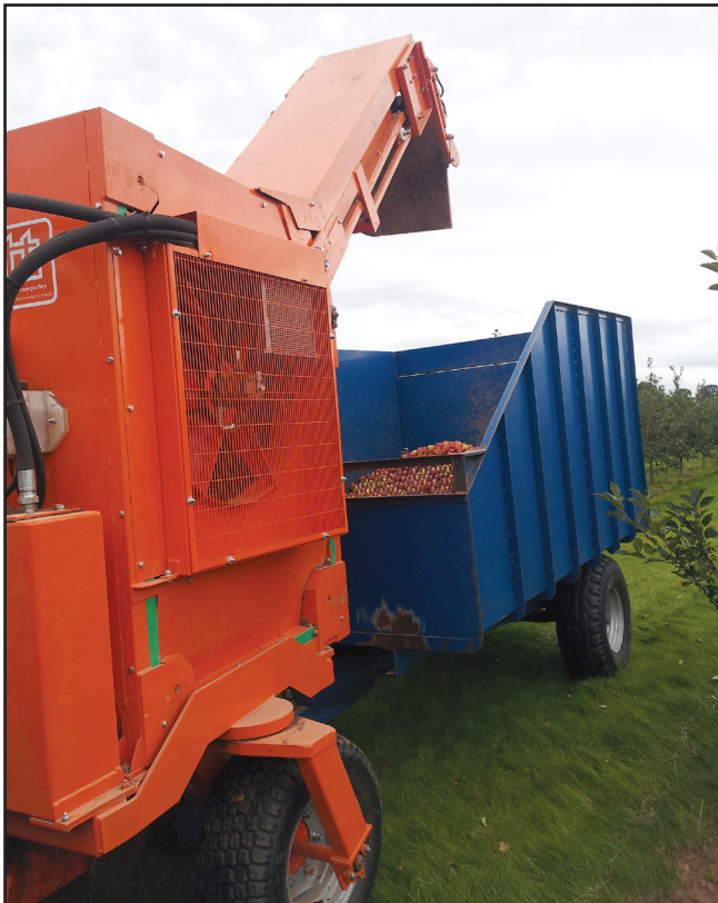
Superb cleaning in any conditions with a long wide hedgehog cleaner belt and a powerful fan
