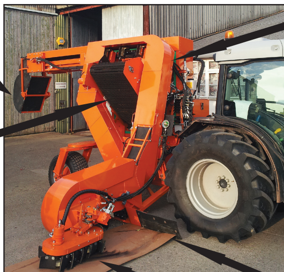
Tuthill Centipede Head Sweep - folds out for the wider rows and back in narrow rows
